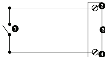
Figure 5.1 N.O. - Normally Open Non-supervised Connections
